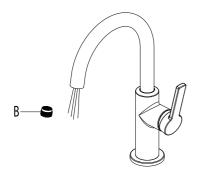
After installing faucet, remove aerator (B) with a coin. Turn water on for 30 seconds to remove any debris. Reassemble aerator (B).
